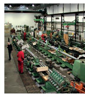
The fabrication of boat shafts requires large, sophisticated machinery to maintain the tight tolerances necessary. © Schaffran Propeller + Service GmbH
