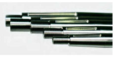
Boat shafts require precise machining of the taper where the propeller is attached.  $\ensuremath{\textcircled{}}$  Clements Engineering
