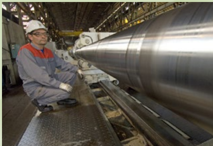
Long dimensional machining
