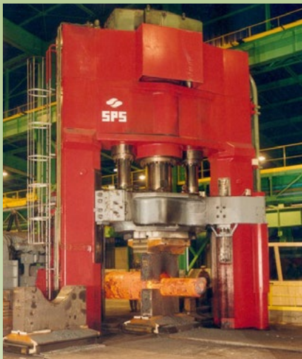
4500 T forging press
