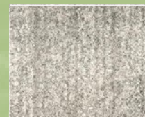
Fine and isotropic microstructure (x100)
